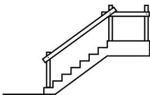
**Wall type and construction:** Depending on wall material and construction type it is sometimes advisable to add additional support within the wall cavity for fixing of the string to the wall. Specific guidance should be sought from the building designer in collaboration with the stair manufacturer at the design stages of the project. This will also help to ensure that CDM Requirements are met.
